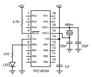
Build and double check this simple circuit on a breadboard and plug in the PICmicro you just programmed. Our line of **PICProto** prototyping boards is perfect for this kind of thing.
