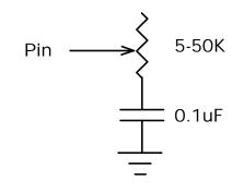
**POT** 3,255,B0 Serout 0,N2400,[#B0] ' Read potentiometer on Pin3 to determine scale ' Send pot value serially out Pin0
