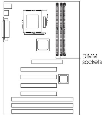
The CB60-BX system board is equipped with three 168-pin DIMM (Dual In-line Memory Module) sockets that support x64/x72 unbuffered or registered PC SDRAM DIMM, 3.3V.
