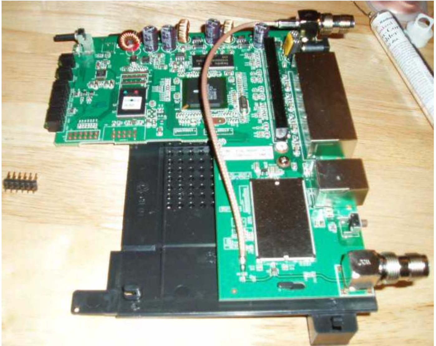
Turning upside-down the router and the 12-pin header being held in place by a plastic cap for my tube of solder.
