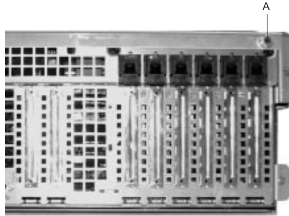
Figure 2. One of Two Thumbscrews Securing Top Cover
