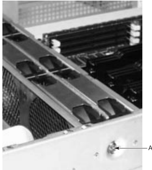
Figure 30. One of Two Screws Securing the Fan Board Assembly
