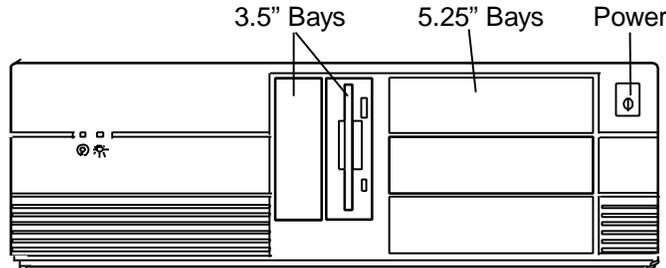
Figure 5: Premiere/PCI Expandable Desktop Front Panel
