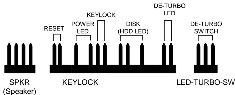
Figure 3: Front Panel Connectors
