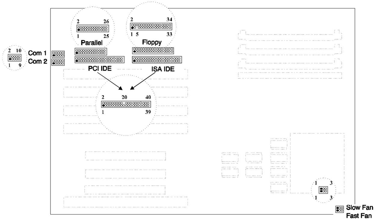
Figure 4. I/O Connections
