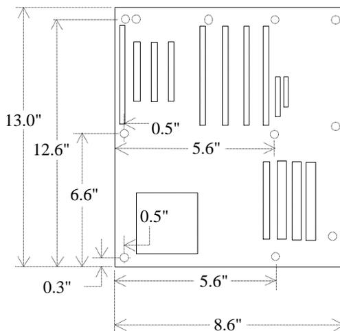
Figure 1. Premiere/PCI Baby-AT Motherboard dimensions.
