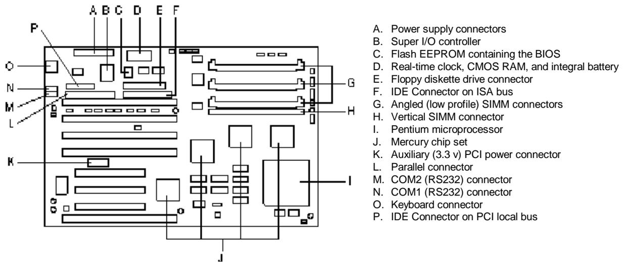
Figure 2. Premiere/PCI Baby-AT Motherboard components
