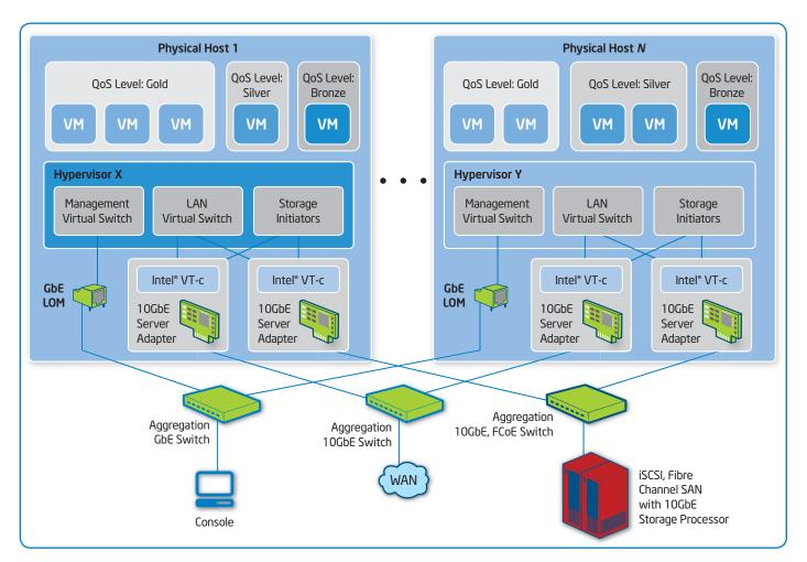
Figure 5. Network policy, traffic shaping, and scheduling enable robust quality-of-service support.
