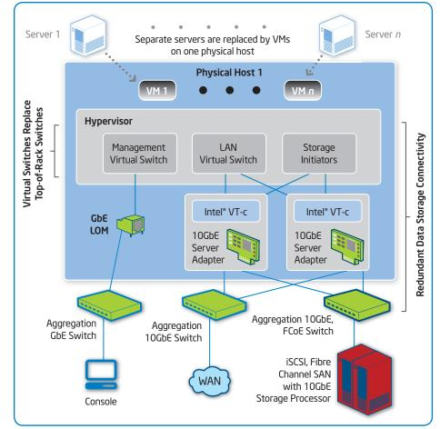
**Figure 3.** Intel<sup>®</sup> Virtualization for Connectivity offloads switching and sorting from the processor to the network silicon, for optimized performance.
