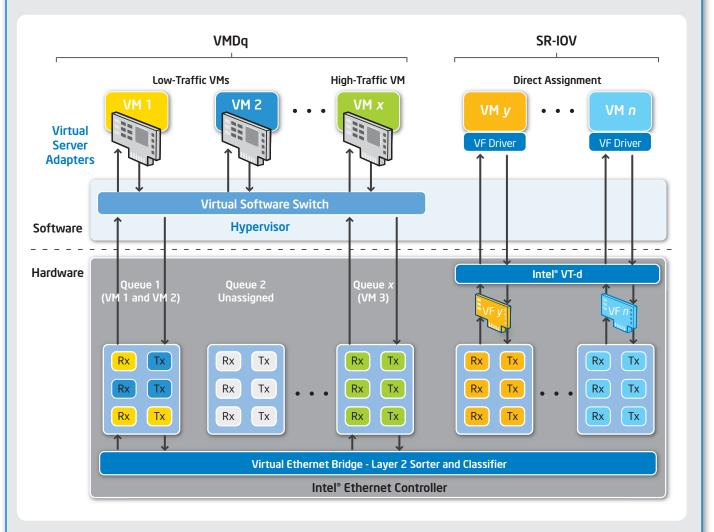
Figure B. Intel<sup>®</sup> VT-c supports I/O virtualization with both VMDq and SR-IOV, both of which enhance network performance dramatically for cloud environments.
