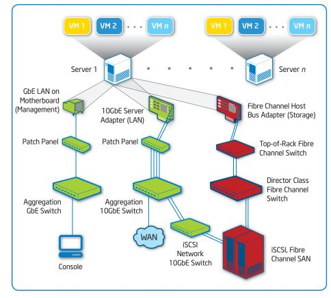
Figure 1. Consolidating Gigabit Ethernet (GbE) server adapters onto 10GbE reduces the number of ports and cables in the network, lowering complexity and costs.
