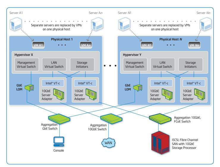
Figure 4. Intel® Virtualization for Connectivity supports combinations of all major hypervisors in the same environment by providing both Virtual Machine Device Queues and Single Root I/O Virtualization support.
