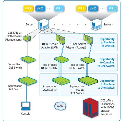
Figure 2. Intel<sup>®</sup> Ethernet 10GbE Server Adapters support storage technologies, such as NAS (Network Attached Storage), iSCSI (Internet Small Computer System Interface), and FCoE (Fibre Channel over Ethernet), enabling both storage and LAN traffic to be passed over Ethernet.
