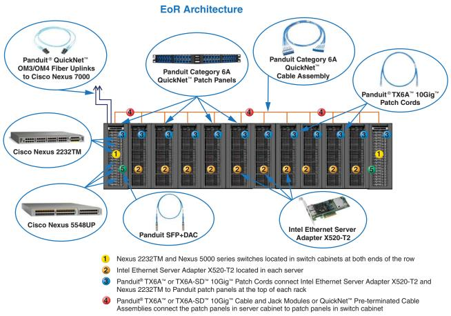
5 Panduit SFP+ passive Direct Attach Copper cables connect Nexus 2232TM to Nexus 5000
