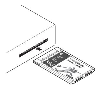
Inserting the CardBus into the Computer
