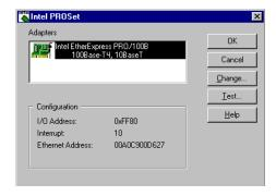
PROSet is an enhanced utility that you can use to easily configure and test your adapter in Windows NT. PROSet also displays the computer resources that were assigned to each PRO adapter installed.
