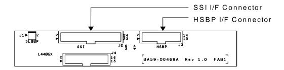
Figure 11. Connectors in Front Panel
