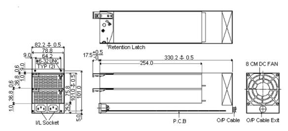
Figure 5. Outline Drawing Power System Enclosure
