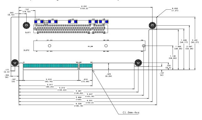
Figure 18. Component and Connector Placement of Rigid Printed Circuit
