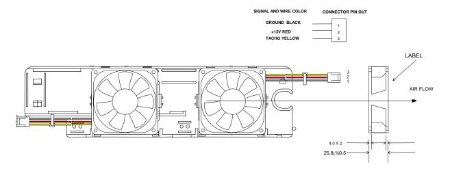
Figure 9. 80-mm Mid System Fan
