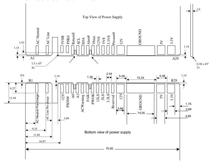
Figure 7. Power Supply Module Edge Connector
