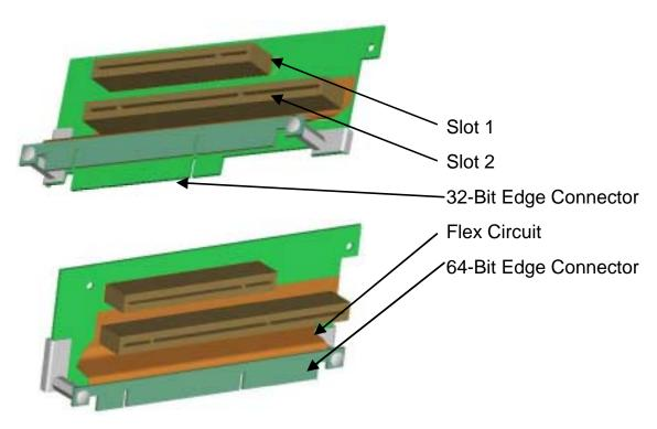
Figure 17. PCI Riser for STL2 Component and Connector Description
