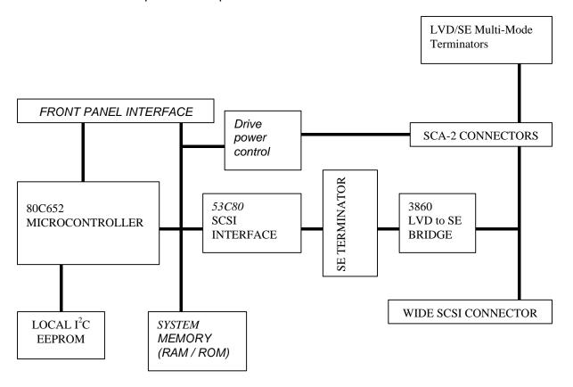
Figure 14. HSBP Functional Block Diagram
