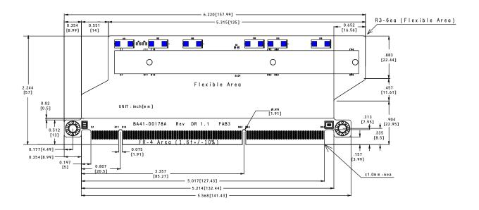
Figure 19. Component and Connector Placement of Flexible Printed Circuit
