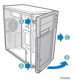
Figure 16. Removing Bezel
