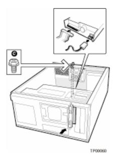
Figure 8: Drive Bay Locations for Server Chassis SC5275-E
