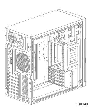
Figure 5. Rear Internal View of the Intel® Server Chassis SC5275-E
