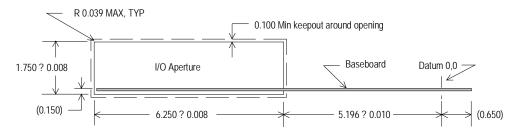
Figure 1. ATX 2.2 I/O Aperture
