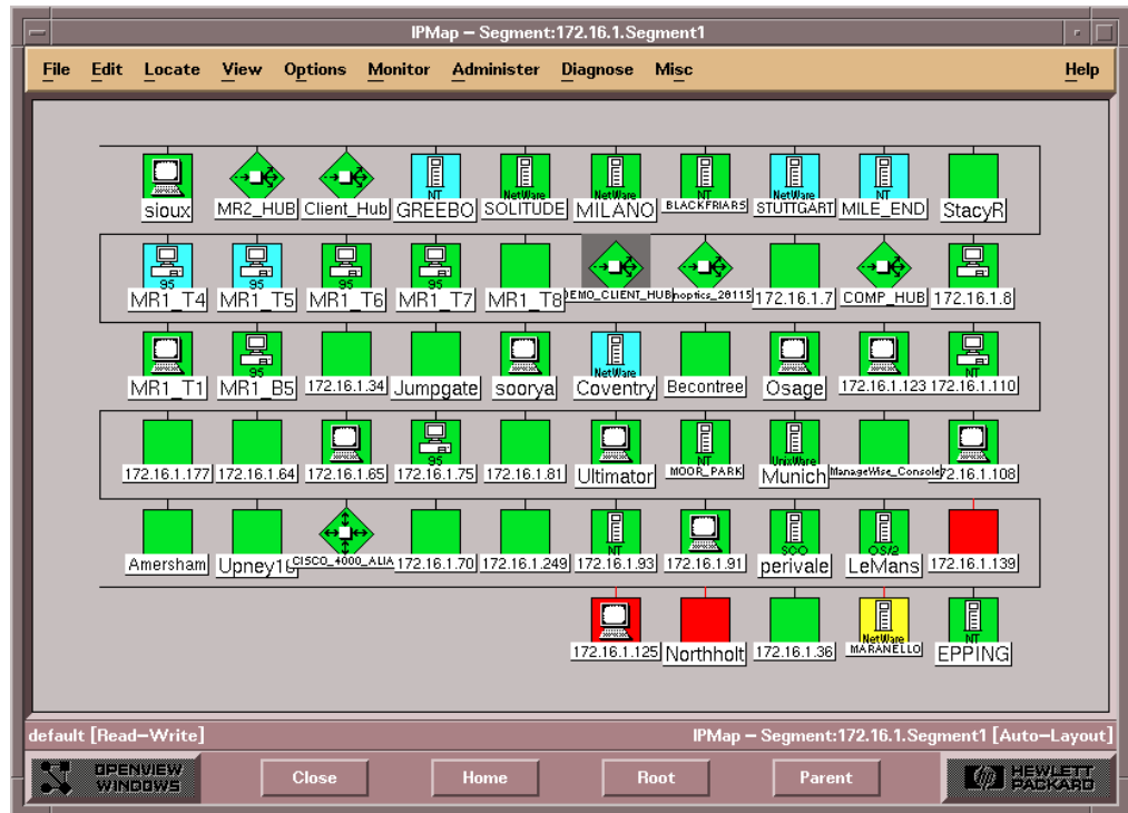
Figure 2 - Compaq Insight Manager for OpenView integration at the Segment Sub Map of OpenView
