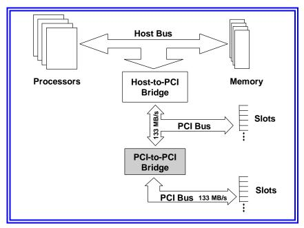
Figure 5: PCI-to-PCI bridge architecture.
