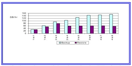
Figure 7: Performance of IntranetWare backups and restores by numbers of SCSI cards in relation to numbers of tape drives (shown at the bases of the columns).
