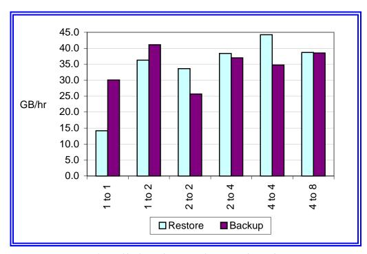
Figure 9: Local backup and restore performance under Windows NT with various proportions of SCSI cards and 35/70 GB DLT drives (shown at bases of columns).
