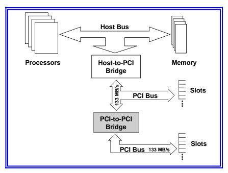
Figure 5: PCI-to-PCI bridge architecture.
