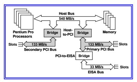
Figure 4: ProLiant 5000 peer-to-peer bus architecture. The ProLiant 5000 has seven PCI slots and three EISA slots across the two PCI buses (eight total; two are shared).
