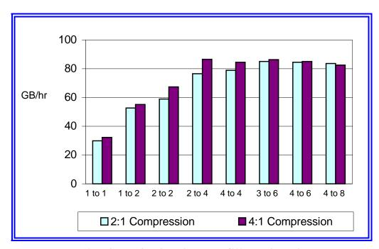
Figure 10: Backup speed results on the ProLiant 6000 test under Windows NT, with various proportions of SCSI cards and 35/70 GB DLT drives (shown at bases of columns).
