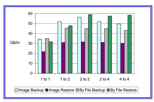
Figure 6: Performance results from tests comparing various proportions of 53c875 SCSI cards to DLT drives (shown at the bases of the columns).
