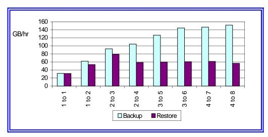
Figure 7: Performance of IntranetWare backups and restores by numbers of SCSI cards in relation to numbers of tape drives (shown at the bases of the columns).
