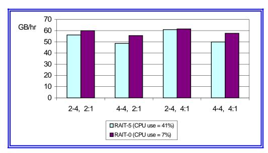
Figure 13: RAIT-5 and RAIT-0 performance with various proportions of cards to drives and two compression ratios (shown at bases of columns).
