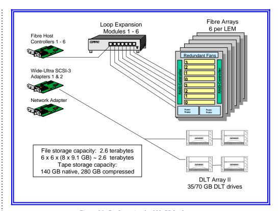
Figure 16: Configuration for 800-GB backup test.
