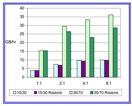
Figure 12: Data compression effects at various levels of compression (indicated at bases of columns).
