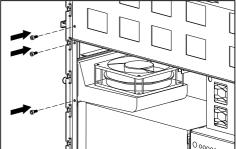
Figure 6. Three set screws mounted on the chassis under the side panel are provided for optional use to lock rear-mounted, quick release modules in place. If moved to the indicated positions, these three screws will secure the processor module, the I/O module, and the fan against quick release and removal.
