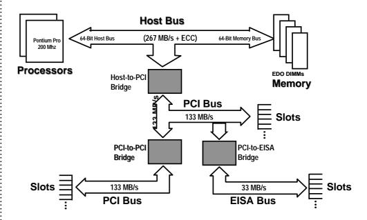
Figure 11. Block diagram showing the PCI-to-PCI bridge architecture used in the Compaq ProLiant 2500 Server.
