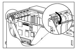
Figure 4. In a ProLiant 2500 tower model, PCI and EISA cards slide into the I/O slots from the top (left). A unique rotating latch secures each card (right).
