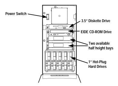
Figure 10. Front view of the Compaq ProLiant 2500 Server chassis showing four removable media bays and a hard drive cage containing five 1-inch hot-plug drives.
