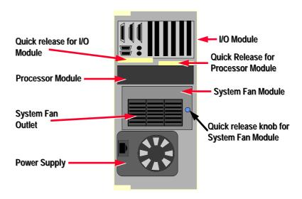
Figure 3. Rear view of the ProLiant 2500 Server chassis showing lever-actuated quick release modules.
