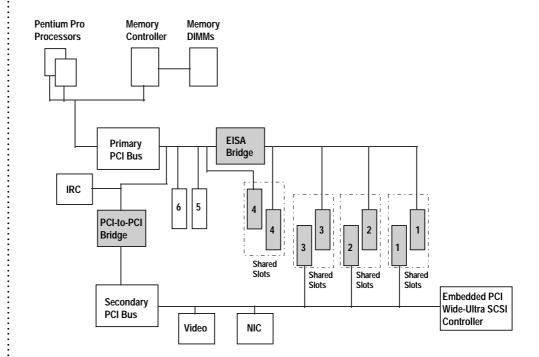
Figure 12. I/O Architecture of the Compaq ProLiant 2500 Server.
