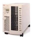
The ProLiant 5500 supported up to four 550- or 500-MHz Pentium III Xeon processors with 100-MHz front-side bus and full-speed cache. The 5500 shipped with 512-K or 1-MB L2 cache with 2 MB optional. The dual-peer PCI architecture eliminated the need to balance I/O. The system shipped with 256 MB of ECC EDO memory expandable to 4 GB using industry-standard DIMMs. The system supplied seven expansion slots, including six PCI and one shared PCI/ISA slot.
