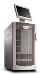
A multi-node system, the Compaq ProLiant Cluster for NetWare 5 uses NetWare Cluster Services (NWCS) to supply high levels of uptime for business-critical services. This solution provides up to an 8-node all-active cluster support meaning that any NetWare server in the cluster can restart resources from a failed server as well as single point administration through the Novell Console One cluster configuration and monitoring GUI.
