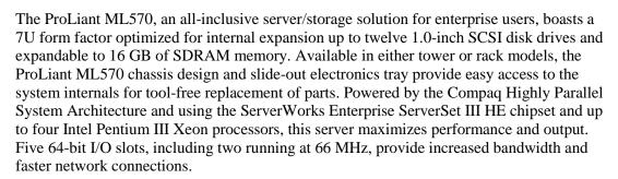
High availability features include hot-plug redundant fans, power supplies, NICs, and drives in addition to new memory error correcting technology built into the chipset. The ProLiant ML570 ships with a Compaq NC3123 Fast Ethernet PCI 10/100 WOL NIC and an integrated dual-channel Wide Ultra2 SCSI Adapter.
