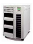
The ProLiant 6000 delivered breakthrough enterprise performance and the highest levels of expansion for the best value in business-critical environments. The ProLiant 6000 offered up to four 500-MHz Pentium III Xeon processors providing industry-leading performance for CPU-intensive applications, such as Windows NT Terminal Server and database applications. The ProLiant 6000 provided leadership performance and unparalleled expansion in an easy-to-service, industry-standard platform.
