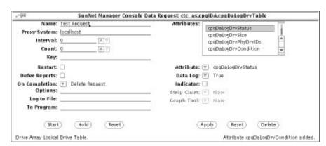
**Figure 5-6.** Requesting a data report for logical drive information on a drive array
