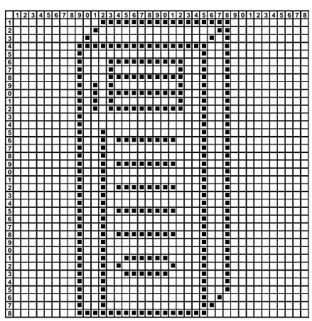
Figure 4-1. Bitmap for a Compaq server (38 x 38 pixels)
