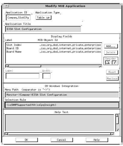
**Figure 6-3.** Building an application for EISA configuration information
