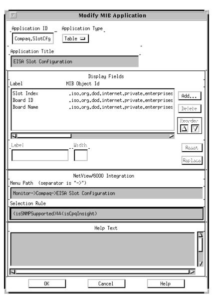
**Figure 4-3.** Building an application for EISA configuration information
