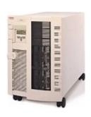
The ProLiant 5500 Server supports up to four 550- or 500-MHz Pentium III Xeon processors with 100-MHz front-side bus and full-speed cache. The 5500 ships with 512-K or 1-MB L2 cache with 2 MB optional. The dual-peer PCI architecture eliminates the need to balance I/O. The system ships with 256 MB of ECC EDO memory expandable to 4 GB using industry-standard DIMMs. The system supplies seven expansion slots, including six PCI and one shared PCI/ISA slot.
