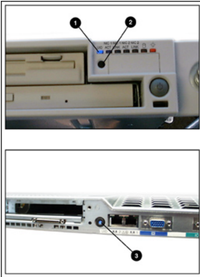
Figure 13: Unit Identification (UID) LEDs and switches on the Compaq ProLiant DL360 server
