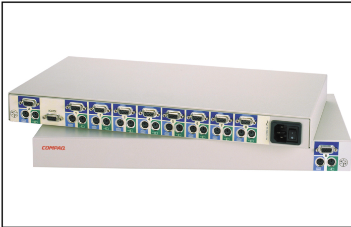
Figure 17: Server Console Switch
