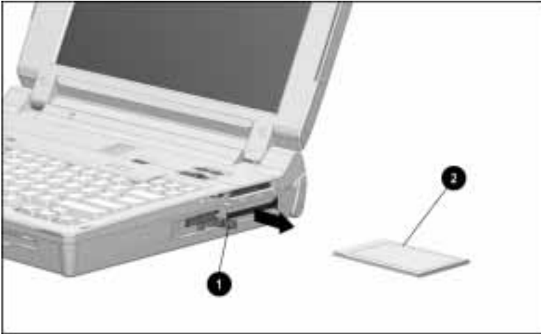
Removing a PC Card
