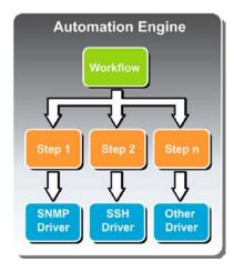
Referring to the diagram above and in relation to the workflows, a driver is a Java class that contains the interface or the protocol code that will interact with the devices in the data center, including the **ThinkControl** service itself.
