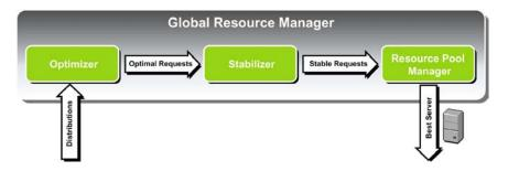
The Global Resource Manager considers the different server requirements for each application environment and then determines where the servers should be allocated. The server reconfiguration and allocation data is then passed to the Deployment Engine, which breaks down the configuration changes into commands that are formatted and sent to the servers and network devices involved to implement the changes.
