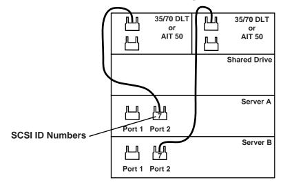
Figure 5: Dual Compaq 35/70 GB DLT Drive or Dual Compaq AIT 50 GB Tape Drive configuration
