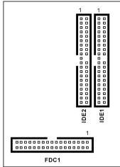
The FDC1 connector connects up to two floppy drives with a 34-wire, 2-connector floppy cable. Connect the single end at the longer length of ribbon cable to the FDC1 on the board, the two connectors on the other end to the floppy disk drives connector. Generally you need only one floppy disk drive in your system.
