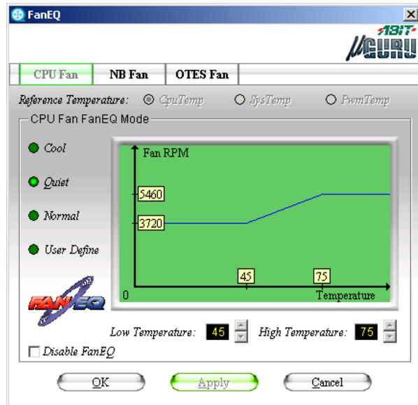
The “CPU FanEQ” controls the speed of the fan connected to “CPU fan header” according to the reference temperature measured from the CPU thermal sensor only.
