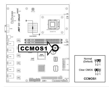
**ATTENTION:** Turn the system power off first (including the +5V standby power) before clearing the CMOS memory.
