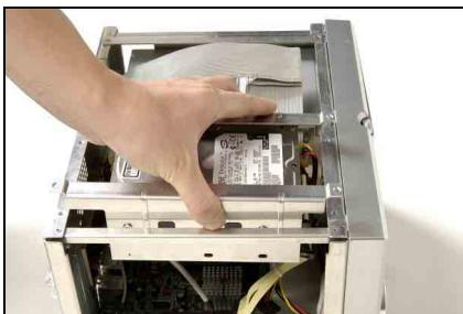
Insert the hard-drive holder vertically down into the chassis.
