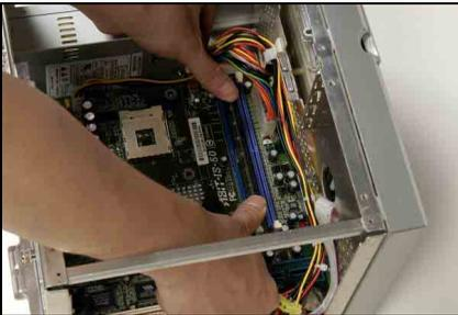
Firmly press the module into the slots by both thumbs until the ejector tabs at both sides of the slot automatically snaps into the mounting notch. Do not force the DIMM module in with extra force as the DIMM module only fit in one direction.
