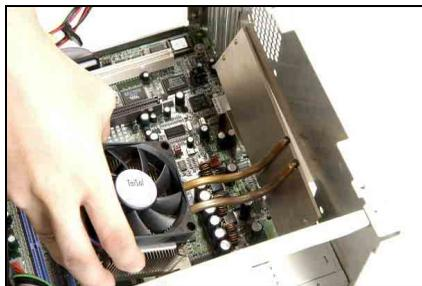
Align the thermal module toward the heat-sinking hole at rear panel.
