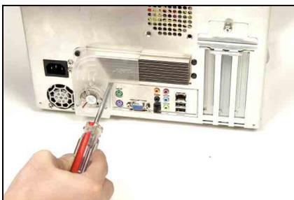
Fasten the screw hole of fan-duct onto rear panel.
