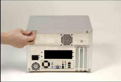
Unscrew the four screws at the rear side of the system chassis by fingers.
