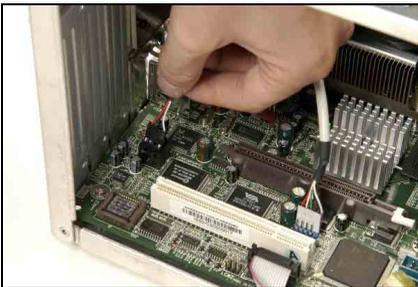
Connect the audio cable from the connector of audio-out on optical-drive to the CD1 on motherboard.
