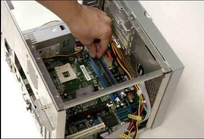
Locate the DIMM slot on the motherboard. Hold two edges of the DIMM module carefully, keep away of touching its connectors. Align the notch key on the module with the rib on the slot. Watch out for the direction, since the module fits in one direction only.
