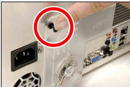
Use one rubber buckle to fasten the fan-duct through the chassis with the external heat sink of thermal module.
