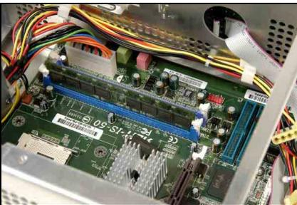
The memory module is firmly installed.
