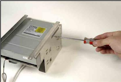
Install one optical drive into the upper layer of drive holder. Fasten the optical drive to the drive holder.
