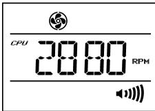
Dial the knob controller clock wise further to view the [CPU Fan Speed].
