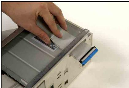
Pass the optical drive cable through the cable hole.
