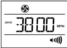
Dial the knob controller clock wise further to view the [System Fan Speed].
