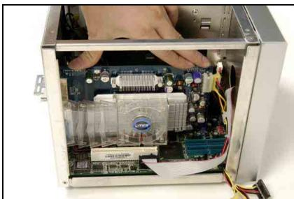
Press down the AGP or PCI add-on card into the slot.
