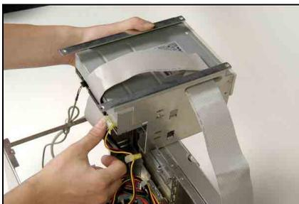
Connect the power cord to optical drive.
