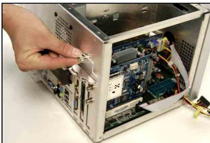
Screw back the I/O shield support by fingers.
