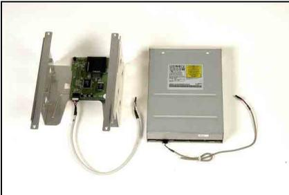
The card reader is already installed beneath the lower layer of the optical drive. Check the signal cable connection.
