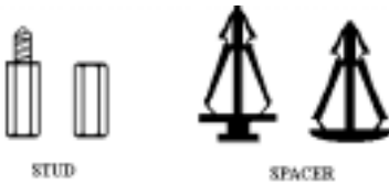
Figure 2-1. The outline of stud and spacer
