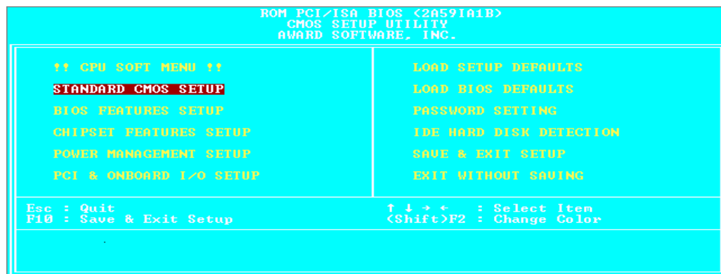
Fig 3 BIOS Setup main menu
