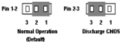
Figure 2-8. CCMOS1 jumper setting
