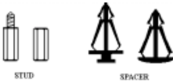
Figure 2-1. The outline of stud and spacer
