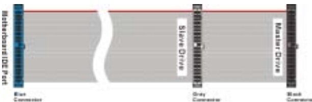
Figure 2-10. Ultra DMA 66 Ribbon Cable Outline
