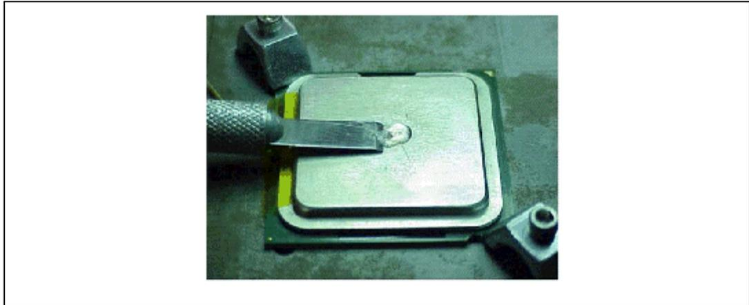
Figure B-13. Filling the Groove with Adhesive
