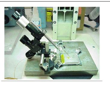
Figure B-9. Measuring Resistance between Thermocouple and IHS
