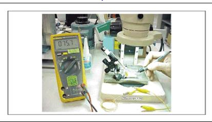
Figure B-10. Applying the Adhesive on the Thermocouple Bead
