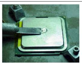
Figure B-13. Filling the Groove with Adhesive
