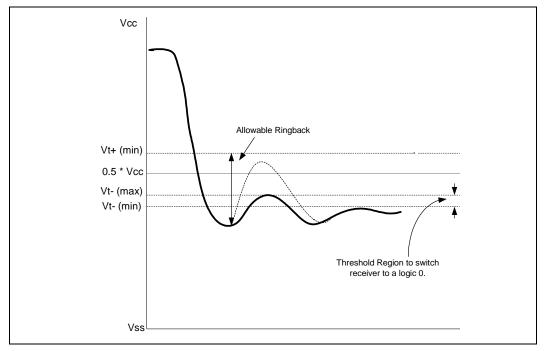
Figure 20. High-to-Low Receiver Ringback Tolerance for TAP Signals
