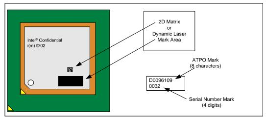
Figure 30. Processor Bottom-Side Markings
