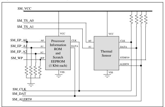
**NOTE:** Actual implementation may vary. For use in general understanding of the architecture. All SMBus pull-up and pull-down resistors are 10K ohms and located on the processor.
