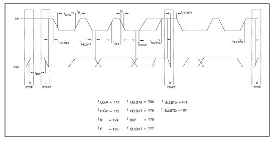
Figure 15. SMBus Valid Delay Timing Waveform
