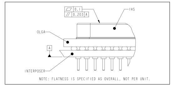
Figure 28. MP Processor IHS Flatness and Tilt Drawing
