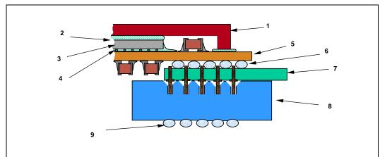
Figure 22. Processor Assembly Drawing (Including Socket)
