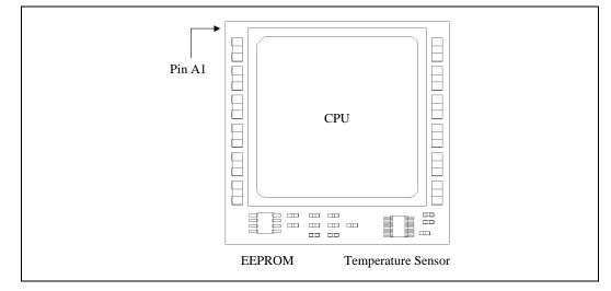
Figure 23. MP Processor Top View Component Placement Detail
