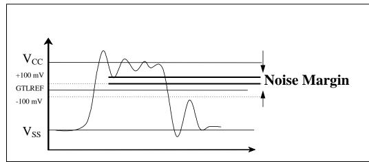
Figure 17. Low-to-High Receiver Ringback Tolerance for AGTL+ and Async GTL+ Signals
