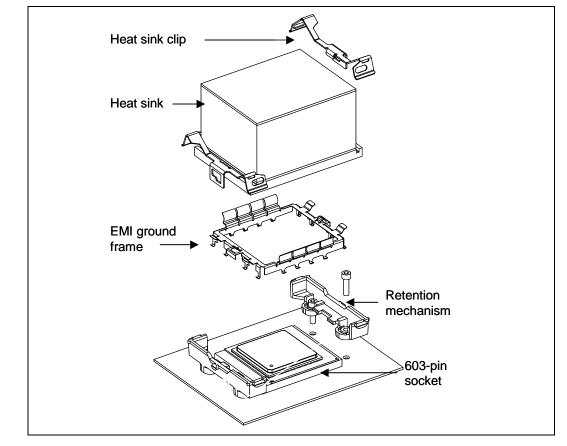
Figure 33. Processor with Thermal and Mechanical Components - Exploded View
