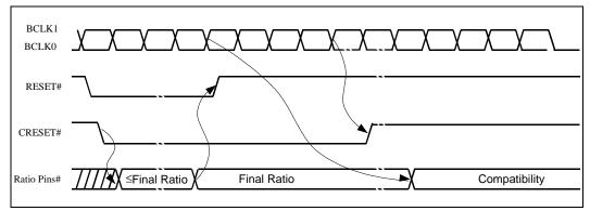
Figure 40. Timing Diagram of the Clock Ratio Signals
