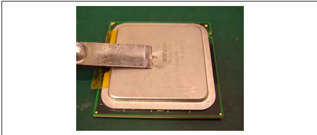
Figure 7-35. Removing Excess Adhesive from IHS
