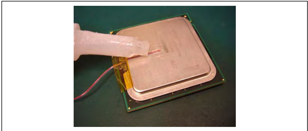
Figure 7-33. Filling Groove with Adhesive
