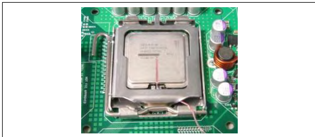
Figure 7-15. IHS Groove at 6 o'clock Exit Orientation Relative to the LGA775 Socket
