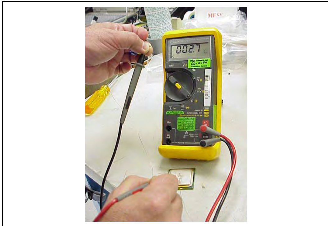
Figure 7-23. Measuring Resistance Between Thermocouple and IHS
