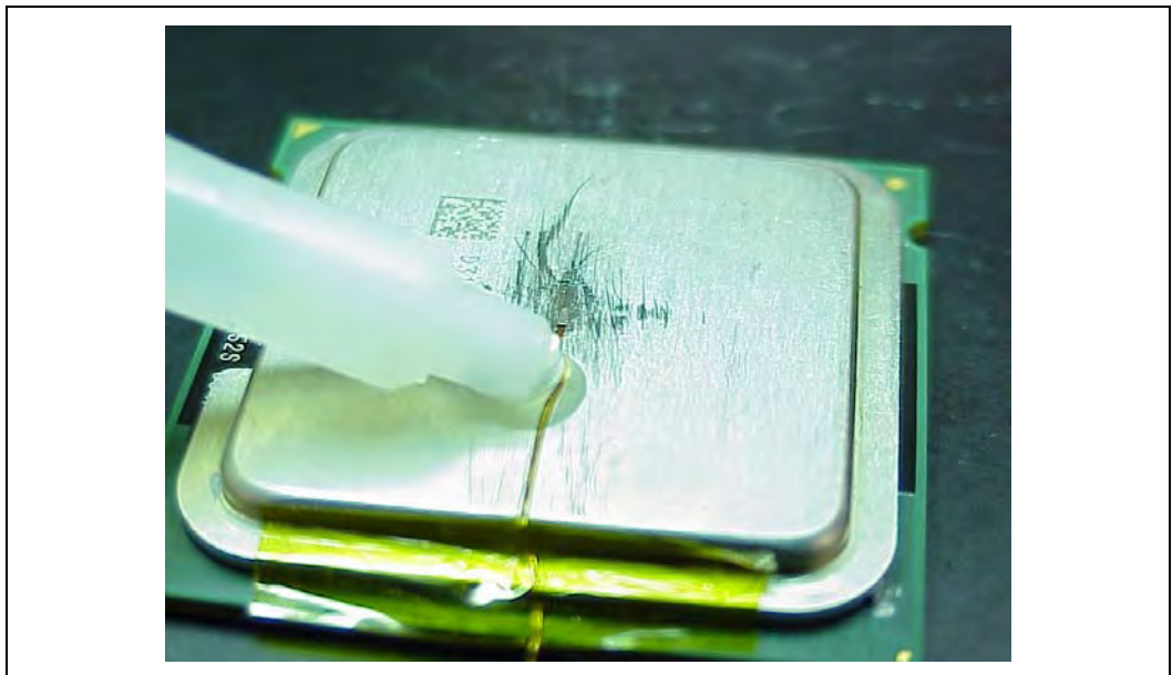
Figure 56. Filling Groove with Adhesive
