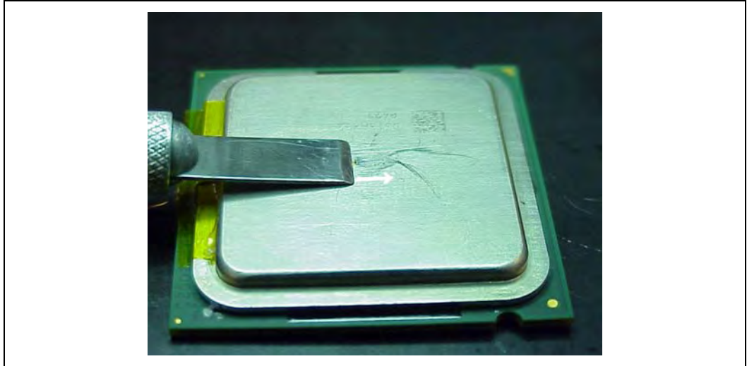
Figure 55. Removing Excess Solder
