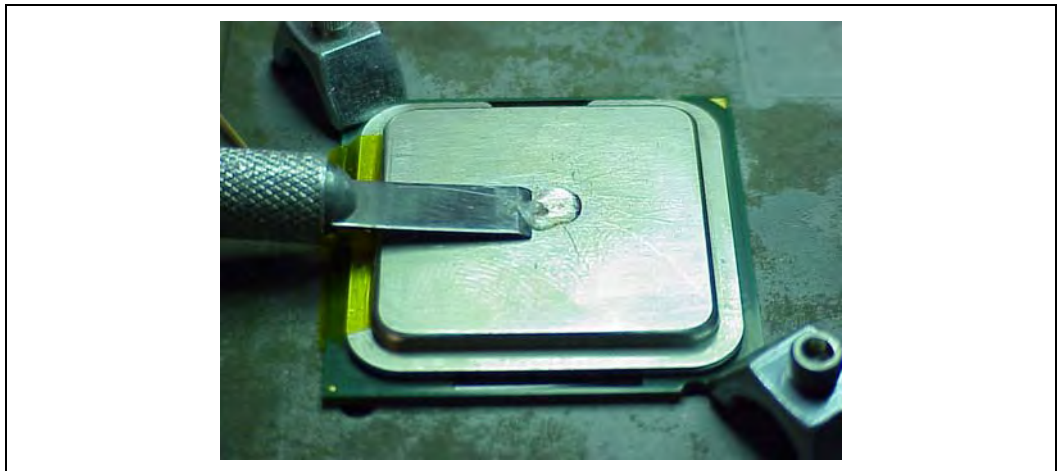
Figure 58. Removing Excess Adhesive from IHS
