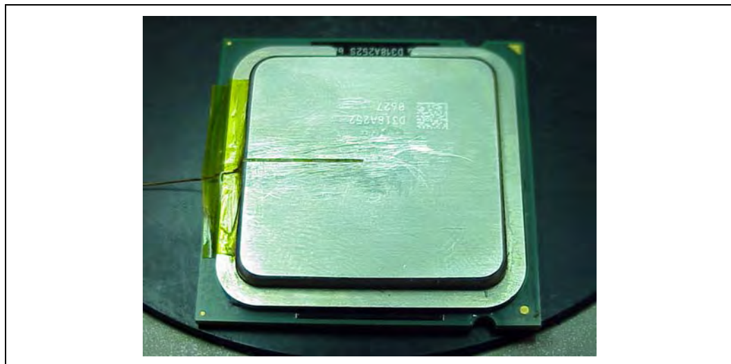
Figure 54. Thermocouple placed into groove
