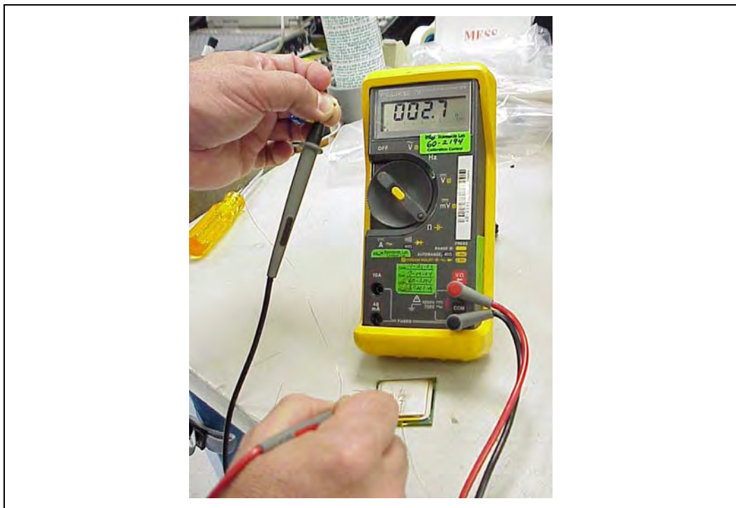
Figure 46. Measuring Resistance between Thermocouple and IHS
