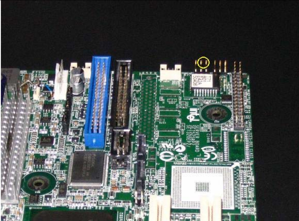
Figure 5. Temperature sensor jumper location
