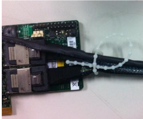
Figure 6. Tie Together the Cables with the Strp Tie
