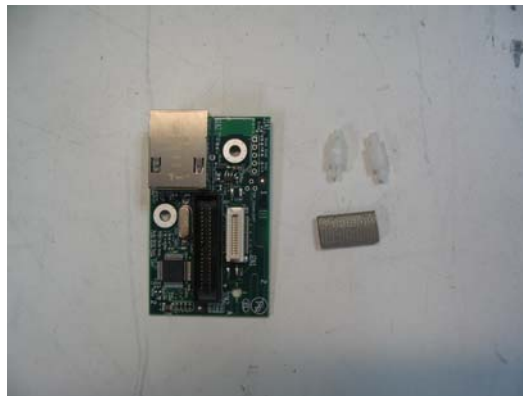
Figure 4 – NIC module, plastic standoffs and EMI gasket
