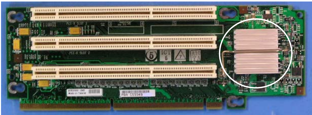
Figure 1: PCI-X Active Riser Card for the Intel Server Chassis SR2400
