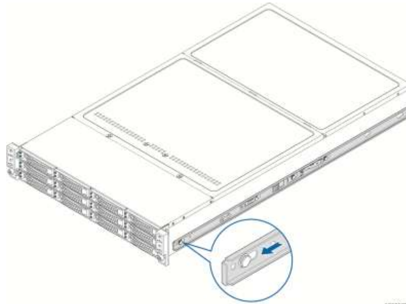
Figure 94. Installing Inner Member of Rail Kit
