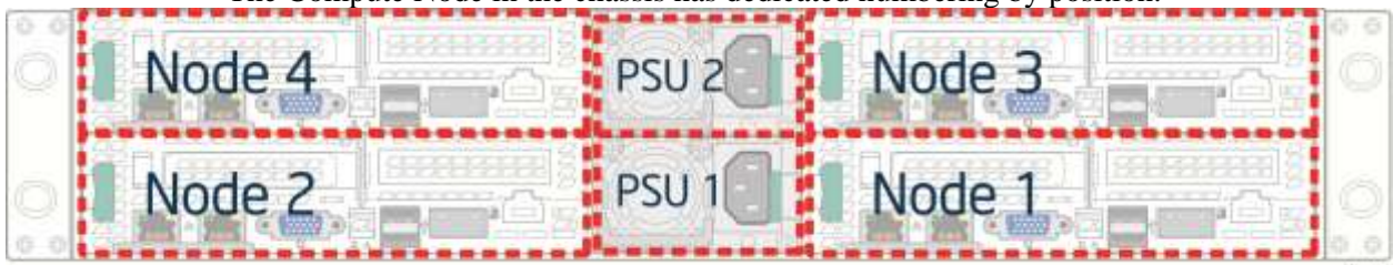
Figure 5. Rear View of Intel® Server System H2000JF with Compute Node Numbering
