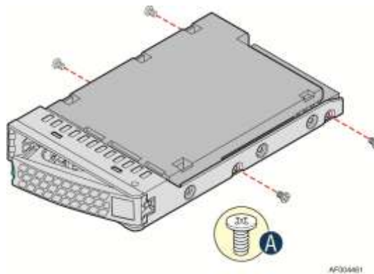
Figure 39. Installing Hard Disk Drive – installing 3.5" HDD to Carrier
