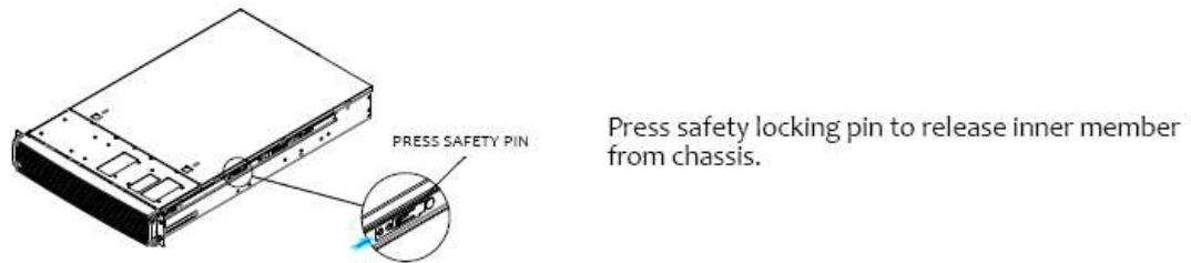
Figure 100. Removing the Chassis from Rack
