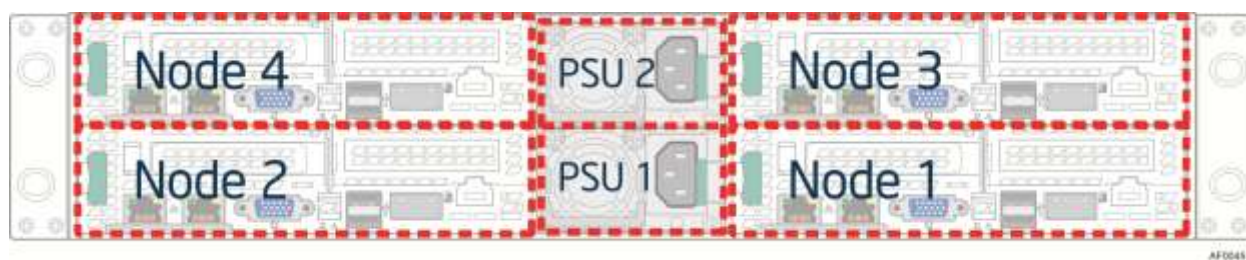
Figure 2. Compute Node Scheme (Rear View)
