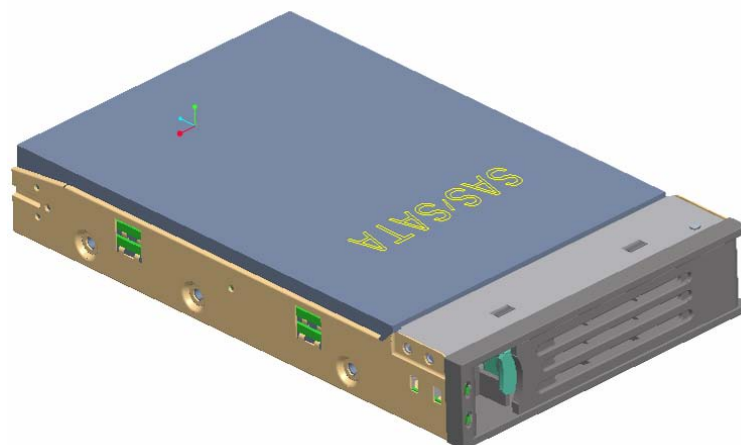
Figure 16. Hot-swap HDD Tray with SAS/SATA HDD Installed
