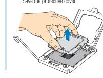
D. Remove the Processor Protective Cover
