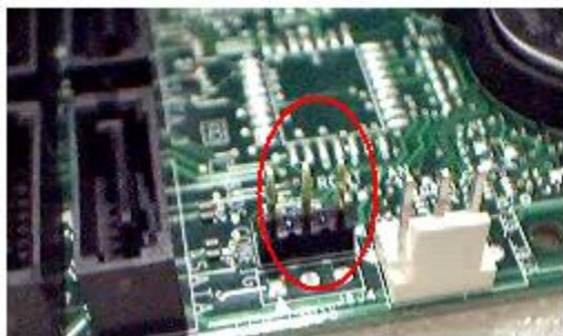
Image 1: Jumper removed (BIOS Recovery Mode)
