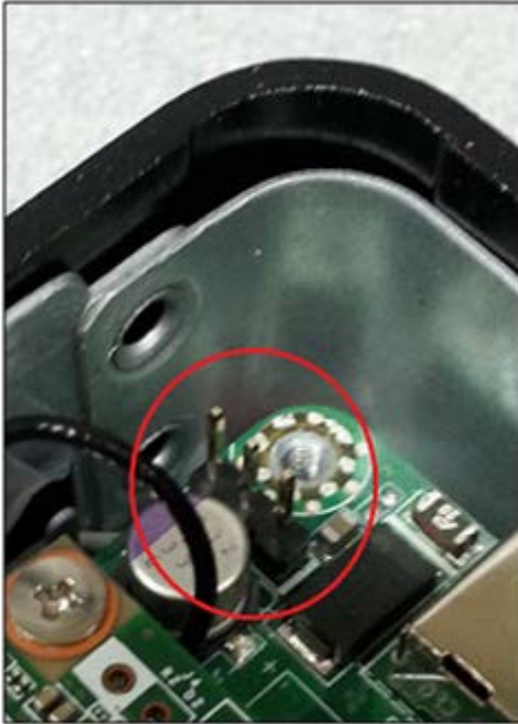
Figure 1: Jumper removed (BIOS Recovery Mode)
