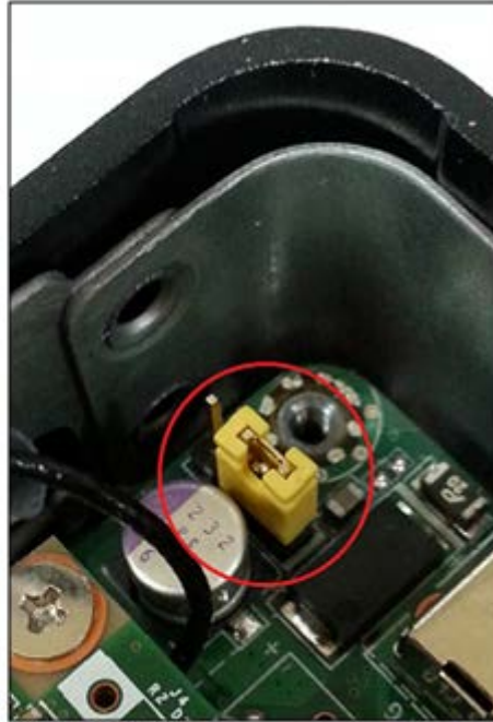
Figure 2: Jumper in place (Normal Mode)
