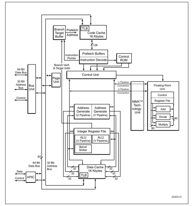
Figure 1. Pentium  $^{\circledR}$  Processor with MMX $^{\intercal}$ M Technology Block Diagram
