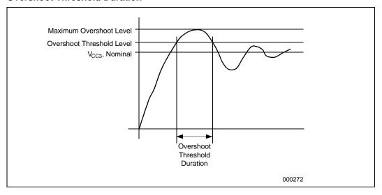
Figure 22. Maximum Overshoot Level, Overshoot Threshold Level and Overshoot Threshold Duration
