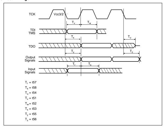
Figure 19. Test Reset Timings
