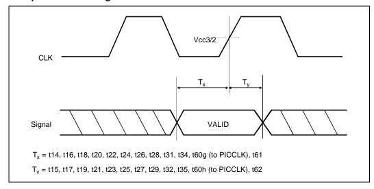
Figure 17. Reset and Configuration Timings
