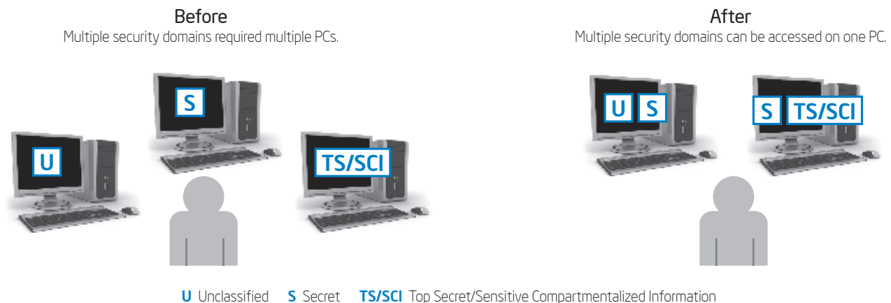
Figure 1. General Dynamics Trusted Virtual Environment (TVE) Desktop* lets workers access networks with different security classifications.
