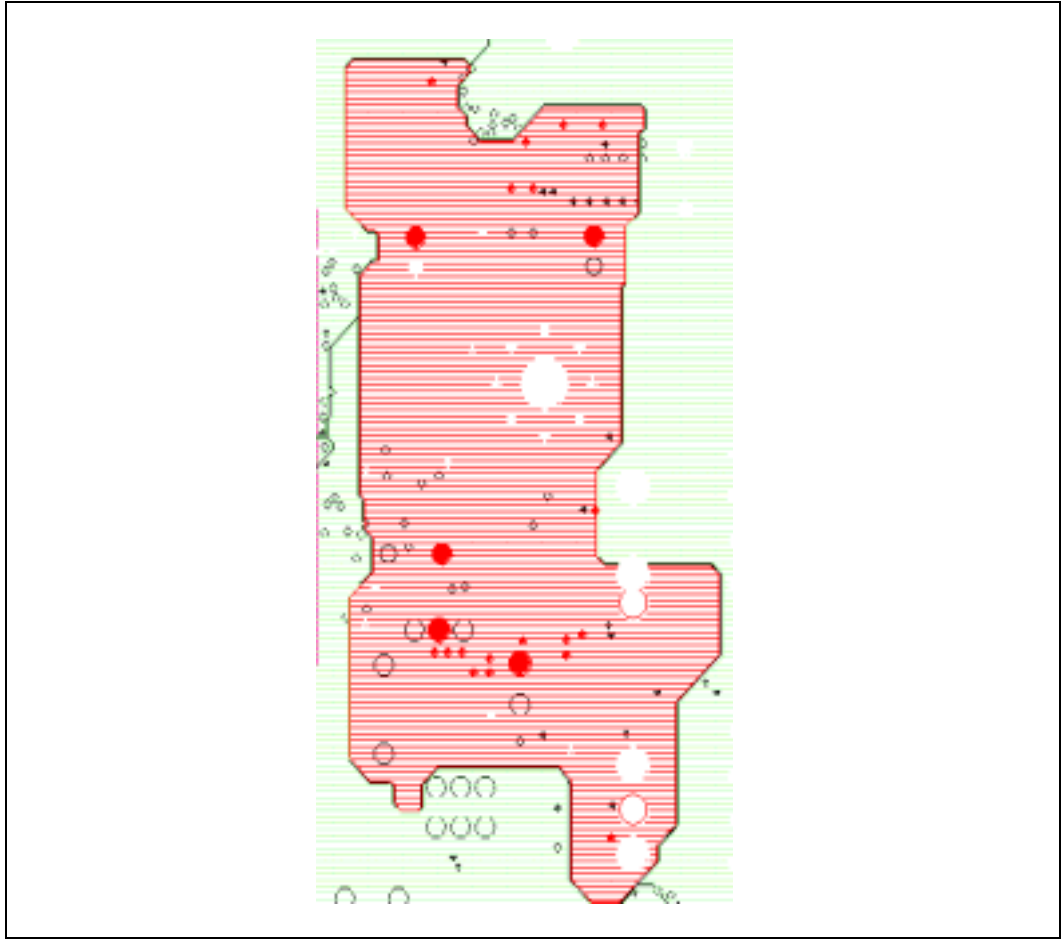
Figure 178. 2.6 V Layer 2 DDR Power Plane
