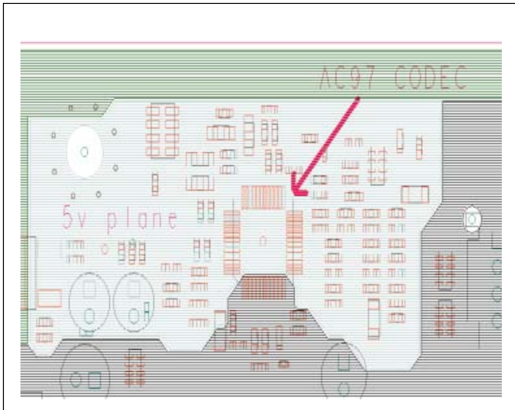
Figure 114. AC '97 Power Plane Configurations
